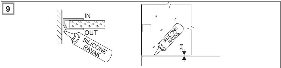
Mount the product into completely finished, tiled bathroom onto the fully fitted bathtub. To ensure the correct functioning, install the product on the fixed walls of the bathrooms only!
